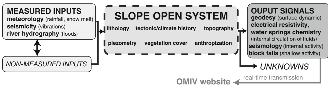
Fig. 4 Conceptual scheme of the different observation components of a slope system
